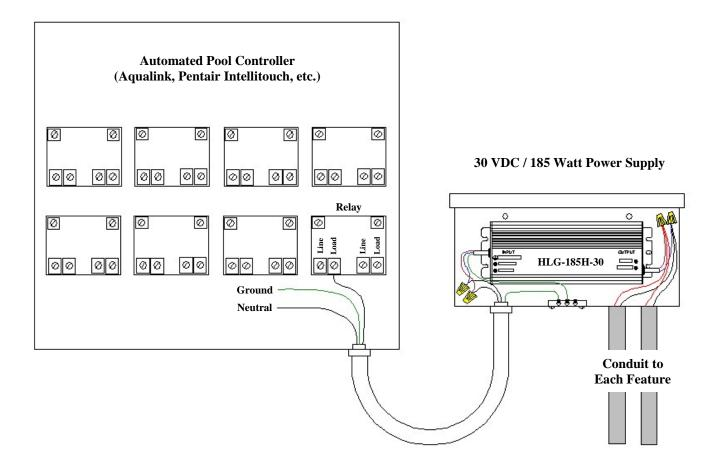
Wiring to Pool Controller when 2 Features Turned ON separately
