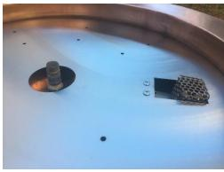
7. Remove the two screws that came with the Burner Pan. Pull the Pilot Burner up through the Opening in the pan and attach it to the pan as shown at right.
