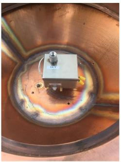
4. On the side of the AWEIS Ignition Control Box there are two brass fittings and two white electrical "Molex" connectors for the Pilot Burner Assembly.
