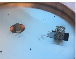
8. Using the cover plates shown at right slip the donut shaped plate over the pipe nipple and the other plate over the Pilot Burner. These plates are meant to be held in place by gravity.
