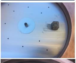
10. Install the burner onto the pipe nipple coming up through the center of the pan.
