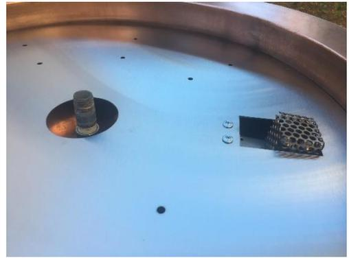
7. Remove the two screws that came with the Burner Pan. Pull the Pilot Burner up through the Opening in the pan and attach it to the pan as shown at right.
