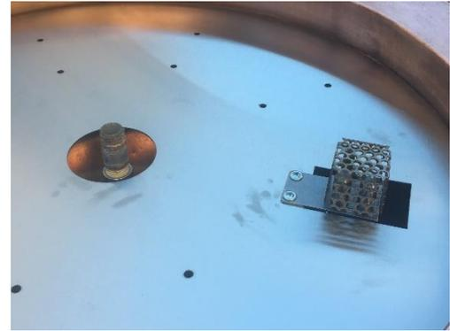
8. Using the cover plates shown at right slip the donut shaped plate over the pipe nipple and the other plate over the Pilot Burner. These plates are meant to be held in place by gravity.
