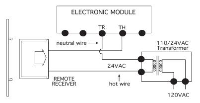
The remote control receiver can be connected, in series, to a 24VAC transformer to the TR (transformer) terminal on the ELECTRONIC MODULE. Connect the hot wire from the 24VAC transformer to either of the wire terminals on the remote receiver. Connect another wire (not included) between the other receiver wire terminal and the TH (thermostat) terminal on the ELECTRONIC MODULE.
