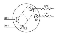
**SPDT SWITCH WIRING**
