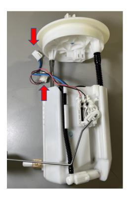
2. Remove the OE retaining clip from the OE top hat support rod (red arrow). Using needle nose pliers pull the retaining clip off.
