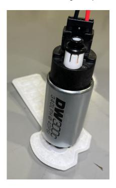
10. Slide the new fuel pump electrical connector through the OE filter assembly (red arrow). Align the DW300c fuel pump outlet with the inlet of the OE filter assembly (yellow arrows). Press the fuel pump firmly into the filter assembly to fully seat the pump.
