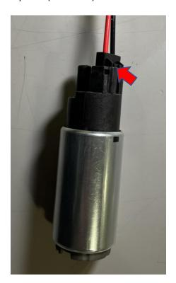
8. Install the new filter sock onto the bottom of the DW300c fuel pump. Align the pump inlet to the large hole on the filter sock (red arrows). Align the filter stud on the bottom of the pump to the small hole on the filter sock (yellow arrow). Press firmly down with the fuel pump onto the filter sock.
