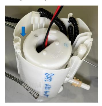
12. Install the OE top hat assembly onto the OE bucket. Verify the OE spring is on the OE top hat support rod (red arrow). Align the support rods into the holes on the bucket (yellow arrows). Install the retaining clip on the bottom of the support rod (Blue arrow).
