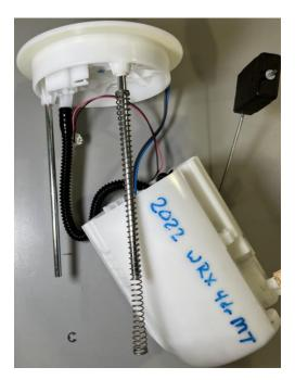
4. Remove the OE center section from the OE bucket. Using small flat head screwdriver release the (3) locking tabs (red arrows). Gently slide the center section out of the bucket from the top.
