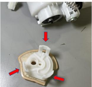
6. Slide the OE fuel pump out of the OE filter assembly. Use a flat head screwdriver to gently push the pump out the bottom of the filter assembly. Remove the OE O-ring from the inside of the filter assembly (red arrow).
