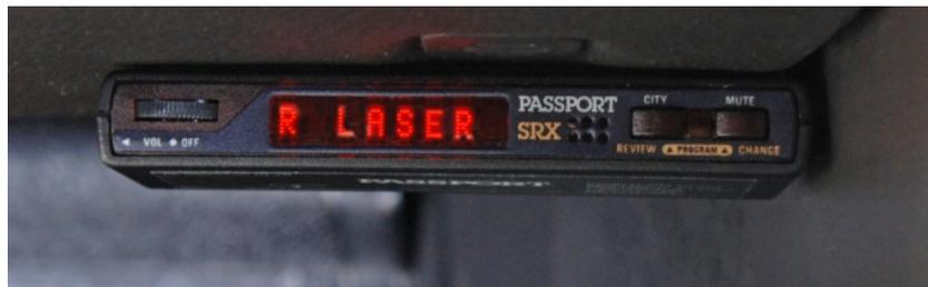
(Code letter E on the installation manual) can be mounted on the lower dash to the right of the steering wheel or buried under the dash or in the center console or anywhere on the HV model after user preferences are programmed if any. **NOTE:** If the owner wants laser shifting enabled this must be performed in programming mode in the Bands MOD selection by setting SHFT in the LSR selection column after all items are completely installed and power is restored.
