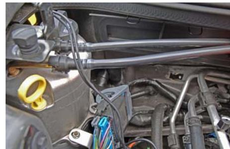
Take a small sharpened 1/8 inch metal rod and poke three holes through the rubber boot. Cut the phone jack connectors off the wires and **run thru the holes in the rubber boot**.
