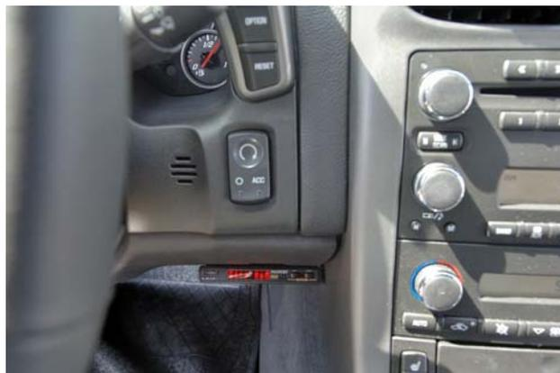
The **Remote Mute Button** (Code letter H on the installation manual) should be located within easy reach of the driver. NOTE: This button has three functions – please consult the owner's manual for explanation.
