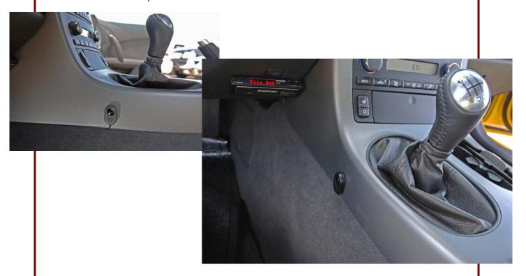
The Bi-Colored Concealed LED Display (optional HV model) can be mounted in the
