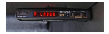
(Code letter E on the installation manual) can be mounted on the lower dash to the right of the steering wheel or buried under the dash or in the center console or anywhere on the HV
