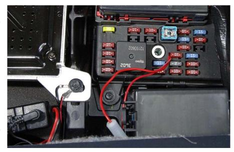
**Display Controller**, Remote Mute / Volume Adjust, Amplified Speaker (Optional HV model), Concealed Display (Optional HV model): All wires from these components will run from the driver side. Feed the wires through the console to the passenger side where the interface is located. The small opening in the console for the wires is located towards the rear of the console. The space is large enough for all wires.
