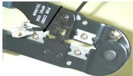
Crimping Too: Mouser Part Number 382-2094C Mouser Electronics, Inc. Phone 800.346.6873 1000 North Main St. www.mouser.com Mansfield, TX 76063 **Step 2**: Place cable in strip part of crimp tool and rotate wire in a circular direction to remove outside jacket. Be sure not to knick the insulation on the separate strand of wire.
