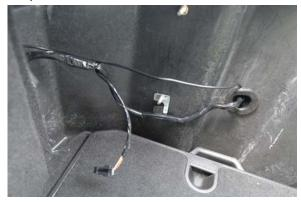
the wire towards the front passenger side to the interface, cut the wire to length, attach a new modular plug and plug the rear laser into the correct interface location.
