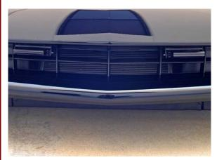
or they can be mounted **outside** the grill using VHB double sided tape as shown on the black car. Spread the shifters as far apart as possible but maintain a clear view of the road ahead. The shifters should be mounted as level as possible (use the sight line on the short side of the shifter as a level line) with the bubble lens on the top of the front face. Remove the protective film from the front face after installation. Feed the wires towards the passenger side of the car under the hood.
