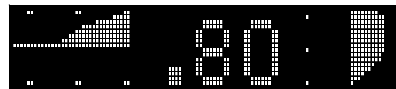
2 seconds later, the car continues to accelerate. (The peak G-Force over the past 4 seconds is .80 G.)
