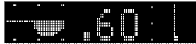
2 seconds later, the car has braked harder, then reduced braking. The car is beginning a right turn. The peak G-Force over the past 4 seconds is .60 G.
