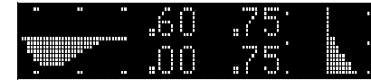
2 seconds later, the car is not braking, but the peak braking G-Force over the past 4 seconds is .60 G. The car is cornering to the right at .75 G.
