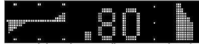
2 seconds later, the car is still cornering to the right, and is beginning to accelerate. (The peak G-Force over the past 4 seconds is .80 G.)
