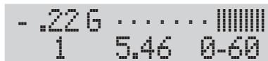
Showing braking of .22G, and a #1 top 0 to 60 run to date of 5.46 seconds.
