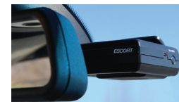
SmartRadar mounted behind mirror
