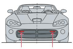
For optimal performance, sensors need to be facing straight forward (or backward, if installing optional rear sensors), not at an angle. Make sure that each sensor is parallel with the road (using supplied bubble level).
