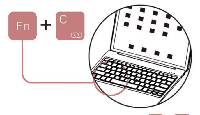
Power on keyboard, then press + keys, the keyboard will stay on searching state within 3 minutes
