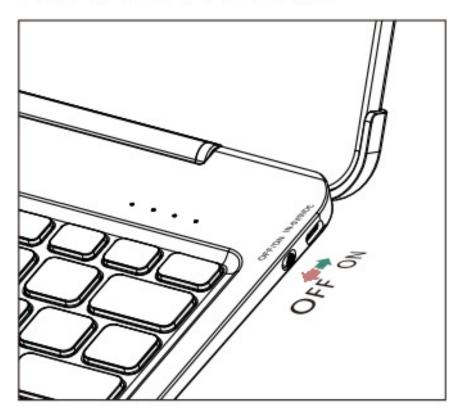
By pushing upward toggle switch to power on the keyboard.
