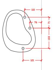
Back to back fixed handles use M8 fixings, which require a 12mm diameter hole glass doors. All handles are handmade, therefore we strongly recommend that doors are marked out and drilled to the physical handle.
