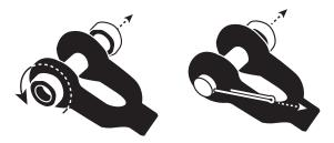
**2** ASSEMBLE TURNBUCKLE BY SCREWING SHAFTS UNTIL EXTENDED AS SHOWN. R WITH R, L WITH L (REVERSE THREADS).
