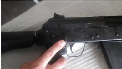
4. Pull the bolt back to the rear via the bolt handle and then release the handle. The bolt will strip a round from the magazine and insert it into the chamber. If the bolt doesn't fully close don't force it closed. Follow unloading instructions if bolt doesn't fully close.
