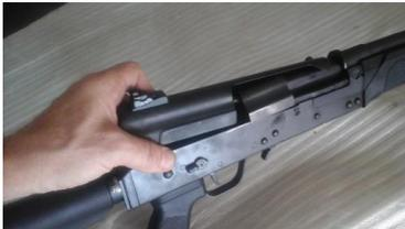
**Step 4:** Push the Upper Receiver Latch forward with your thumb and index finger controlling the latch. Push the latch far enough forward so that it is free of the latch rails and lift up and remove the latch assembly from the receiver... **Be careful because the latch is under spring tension.**
