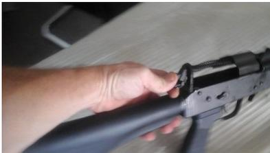
**Step 5:** Disengage safety and then pull bolt assembly to the rear and remove from receiver.
