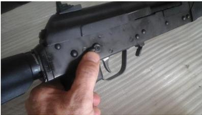
3. To begin firing disengage the safety by rotating it upward, pointing toward "F" make sure you are ready to fire and the shotgun is pointed in a safe direction before you move the safety upward.
