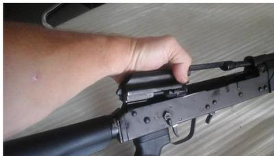
**Step 6:** Separate the bolt from the bolt support, to do this move the bolt backward, give it half a turn counterclockwise and take it out by using a forward motion. To reassemble start with reinstalling bolt assembly and work your way backward through the steps of assembly.
