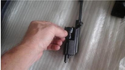
**Step 7:** Access the gas puck. Separate the gas tube stopper. To do this push the spring-loaded plunger flush with a drift pin and undo the stopper with the aid of a screwdriver counterclockwise and withdraw the gas puck.
