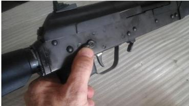
**Step 2:** Depress the Upper Receiver Release Latch button and then depress
