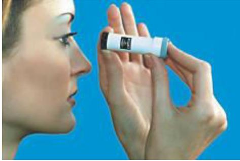
**Fig. 5** Push the optics out of the housing (3) back into the housing and bring the microscope to your eye. With the finger of one hand turn the light on by means of the knob (4.1), and sharpen the picture with the fingers of the other hand by turning the part of the eyepiece (2.1).
