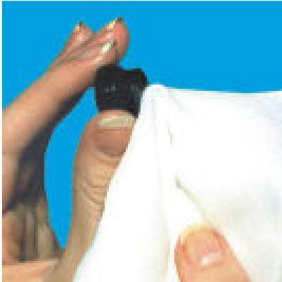
**Fig. 3** Clean softly the glass surface (2.2) of the eyepiece with a clean cloth
