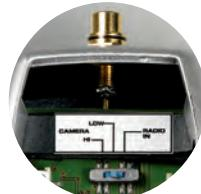
Camera OUT (low or high level) or radio IN switch
