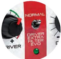
Extra filter even more effective. Moving the switch to "Extra Filter" the background noises are strongly damped and the co-driver voice's louder to the driver. Since the driver's voice sounds lower to the co-driver, it is recommended that the Extra Filter is set to off during transfers.
