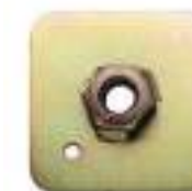
CCM10016 Eye-bolt back plate 65 mm x 65 mm x 3 mm 7/16" UNF thread welded nut, 40 mm 2 . Complies with FIA requirements.
