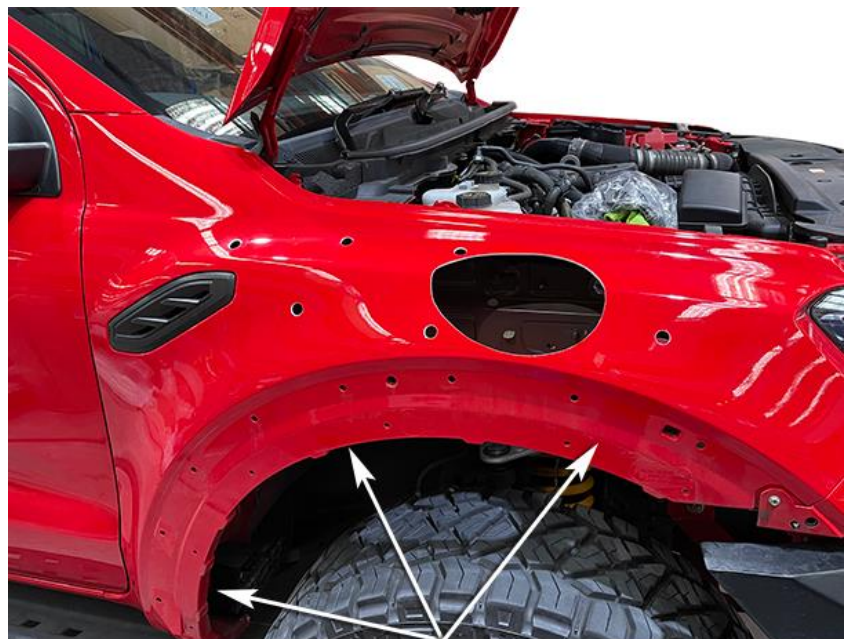
Fender Flare & Inner Guard Liner Removed
