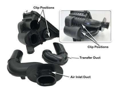
Align and tape the air inlet duct template (item 12) to the air inlet duct flange as shown, mark all hole positions.
