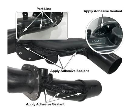
Clean-up any excess sealant to ensure a neat finish.
