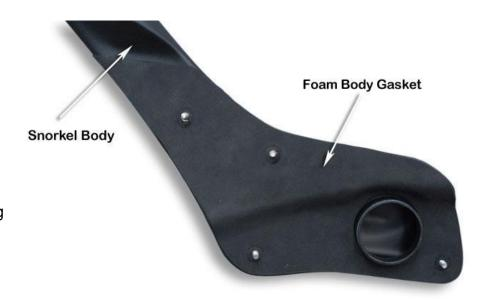
Place a strip of masking tape along the 'A' Pillar panel, carefully install the snorkel body onto the guard panel. Ensure there is adequate clearance around each of the mounting studs.(If necessary enlarge the 16mm mounting holes to achieve adequate clearance around each of the mounting studs to the guard panel using a round file or die grinder).
