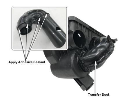
Apply a generous amount of Sikaflex adhesive sealant to the air inlet duct outlet and install the duct into the air cleaner base, ensure the duct clips back into position correctly.
