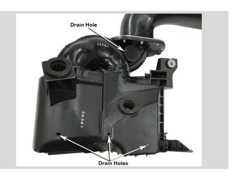
Install the air cleaner base / air entry hose assembly back into the vehicle, guiding the air entry hose through the hole in the inner guard panel as shown.
