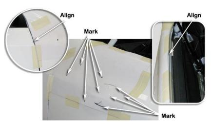
4 Drill a pilot hole for each of the marked hole positions.
