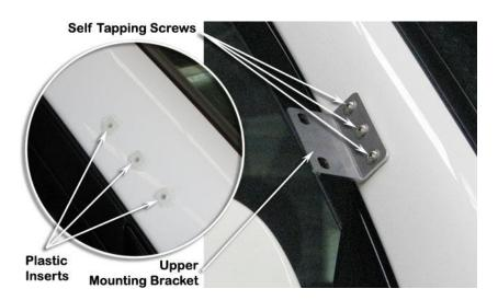
9 Carefully install the snorkel body (Item 1) to the guard panel and align the snorkel body to the guard panel and upper mounting bracket.
