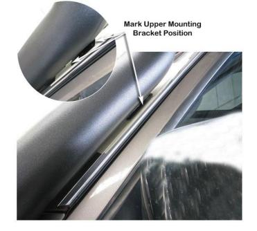
Remove the snorkel body (item 1) from the vehicle and remove the upper mounting bracket (item 3) from the snorkel body.
