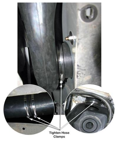
Install the air cleaner element, air cleaner lid and any other components removed during the installation process.
