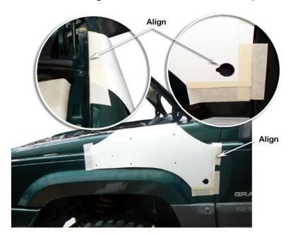
6 Drill a pilot hole for each marked hole position.
