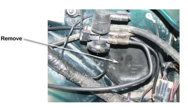
Note: 1993-1995 models must have the PCM moved from the inner fenderwell to in front of the air cleaner assembly (there is plenty of room once the original air intake duct is removed).
