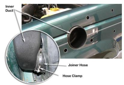
Apply a generous amount of Sikaflex sealant to the outer surface of the snorkel body outlet 26 snout as well as the internal surface of the inner duct to ensure a watertight seal. Carefully guide the snorkel body outlet snout into the inner duct and install the snorkel body to the fender panel.
