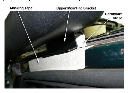
With the snorkel body correctly positioned, ensure the inner duct has adequate clearance between the inner duct inlet and fender panel hole. Mark the upper mounting bracket outline and the four mounting hole positions on the A-Pillar. N.B: The upper mounting bracket edge should be inline with the A-pillar panel.
