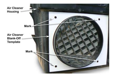
Drill four 5mm (3/16") diameter holes on the positions marked for the blank-off plate.
