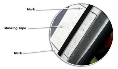
Place the A-Pillar trim back onto the A-Pillar and transfer the upper mounting bracket position to the A-Pillar trim. Extend the length of the markings on the A-pillar trim by approximately 3 mm (1/8") at each end.
