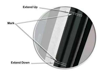
14 Carefully mark the required slot position and drill a 5mm (3/16") hole at each end. Using an hacksaw/air body saw cut a slot in the A-Pillar trim as shown.
