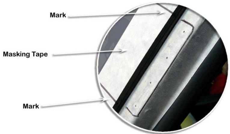
13 Place the A-Pillar trim back onto the A-Pillar and transfer the upper mounting bracket position to the A-Pillar trim. Extend the length of the markings on the A-pillar trim by approximately 3 mm (1/8") at each end. Remove the A-Pillar trim.
