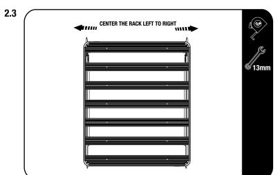
Center the rack left to right using a tape measure. When centered fully tighten the rack to the foot rails starting at one corner and moving to the opposite corner in a criss cross manner. This will keep the rack centered. Fully tighten all remaining bolts.
