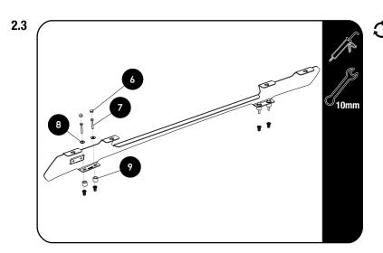
Place sealant over and around the jack nuts to create a watertight seal before placing the spacers over the jack nuts. Place the spacer (Item 9) onto the Jack nut.Fill the tube spacers with sealant.
