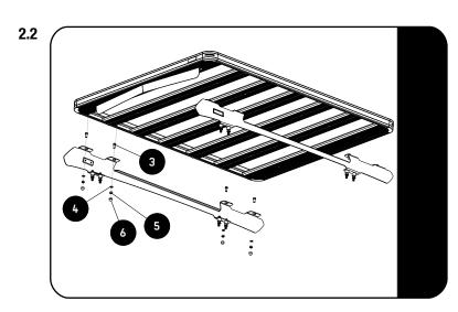
Assemble your roof rack to the Foot Rails using M8x20 hex bolts, M8x16x1.6SS Flat Washers and M8 Nyloc Nuts (Items 3, 4 & 5) as shown.
