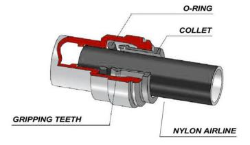
The Push To Connect fitting houses an o-ring and collet to seal and secure the nylon airline.
