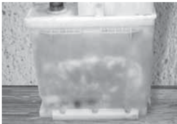
Figure 1 – Picture of battery with deep discharge and sulphation
