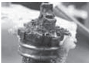
Figure 4 – Picture of a melted battery terminal
