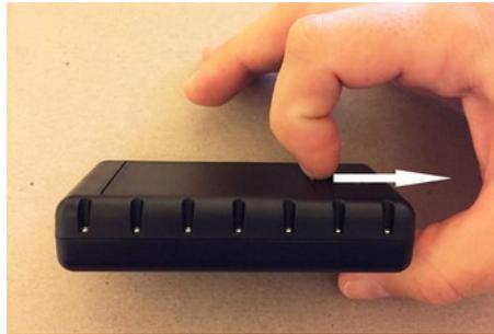
Next, remove battery door to get access to 4 AAA batteries
