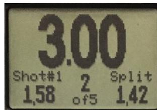
When reviewing shots, pressing the “M” button on front panel once will switch between “single” or “multiple” string viewing mode. Multiple string viewing mode allows you to compare the last 3 strings formatted like a spreadsheet for convenience. At the top are the shot numbers and each row is a string of shots.
