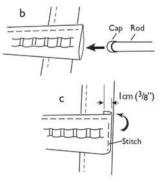
8 Inserting the bottom bar
