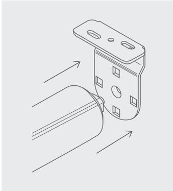
With the Idle pin end in place. Insert the control end into the opposite bracket by depressing the pin end then pull down vertically until the control end clicks into position.
