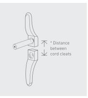
Mark the hole positions and drill as required.
