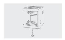
Open the gate of the box brackets and slide the headrail into position then snap the brackets closed.
