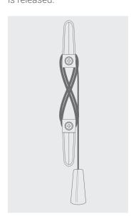
Breakaway safety tassel is pre-fitted to the lift cords so that when a horizontal force is applied to the cords entering the condenser it safely breaks away eliminating any hazardous loops.
