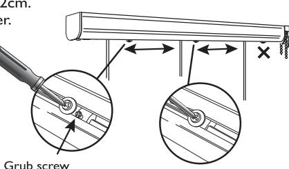
Unscrew & reposition centre guide if needed. Re-secure guides.
