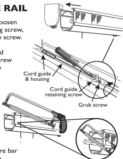
Trim excess rail. When trimming the rail be sure to cut an equal amount from the inside square bar e.g. - trim track 2cm - trim the bar 2cm. Re-attach End cover.
