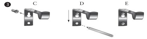
Hook support onto the screw head using the larger key-hole (C). Slide the support downward into position before marking and drilling the bottom support hole (D).
