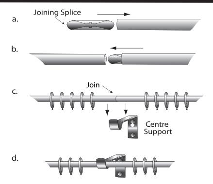
On 240, 300 & 360cm poles. Slide the joining splice into the first pole end(a). Then push the poles together(b). Slide on your rings remembering to leave one at each end as an end stop(c). Position the poles to hide the join behind the centre support(d). Use the allen Key to tighten the grub screw behind the support cup to hold in position.
