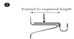
Position support together as shown and fasten securely using the small grub screw.
