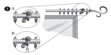
Place the pole into the supports & tighten the screws to hold the pole firmly in place.
