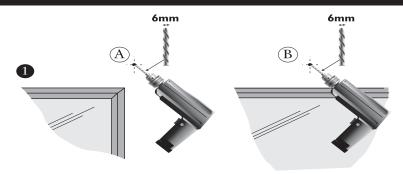
Mark & drill top holes of the support (A) using a 6mm drill bit . On longer length poles mark and drill top hole (B) in the middle for centre support. Fix screw until screw head is approx. 3mm from the wall.
