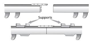
N.B. For strength on longer track, position 1 support either side of the joining bar, this will provide extra stability.
