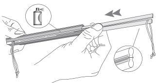
Lightly spray the inside of the track with silicon or furniture polish. Slide both the bending inserts into the track channel ensuring the flat edges are positioned together and the cords are at opposite ends as shown.
