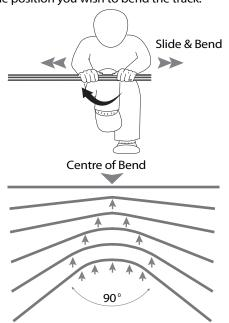
Firmly bend the track in your desired position by applying pressure and Slightly bending and movirting a number of slight bends along the track as above until he desired angle is reached.
