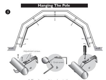
a. Place the complete pole onto the supports. To help align the pole there are some adjustment screws on top of the supports. b. To hold the pole in position, tighten the grub screw underneath with the allen key supplied.  $\emph{c}.$  Finally tighten the adjustment screws on top of the supports.
