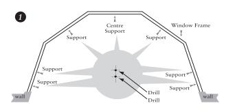
Mark and drill the positions using a 6mm drill bit, for the 7 supports as shown by arrows in the illustration that best matches your window size. Ensure the Centre Support is positioned in the middle of the window, and that the rest of the supports do not interfere with the corner joints. Insert the wall plugs supplied
