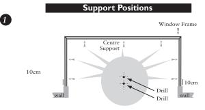
Mark and drill the positions using a 6mm drill bit, for the 7 supports as shown by arrows in the illustration that best matches your window size. Ensure the Centre Support is positioned in the middle of the window, and that the rest of the supports do not interfere with the corner joints. Insert the wall plugs supplied
