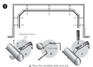
supports. To help align the pole there are some adjustment screws on top of the supports. b. To hold the pole in position, tighten the grub screw underneath with the allen key supplied. c. Finally tighten the adjustment screws on top of the supports.
