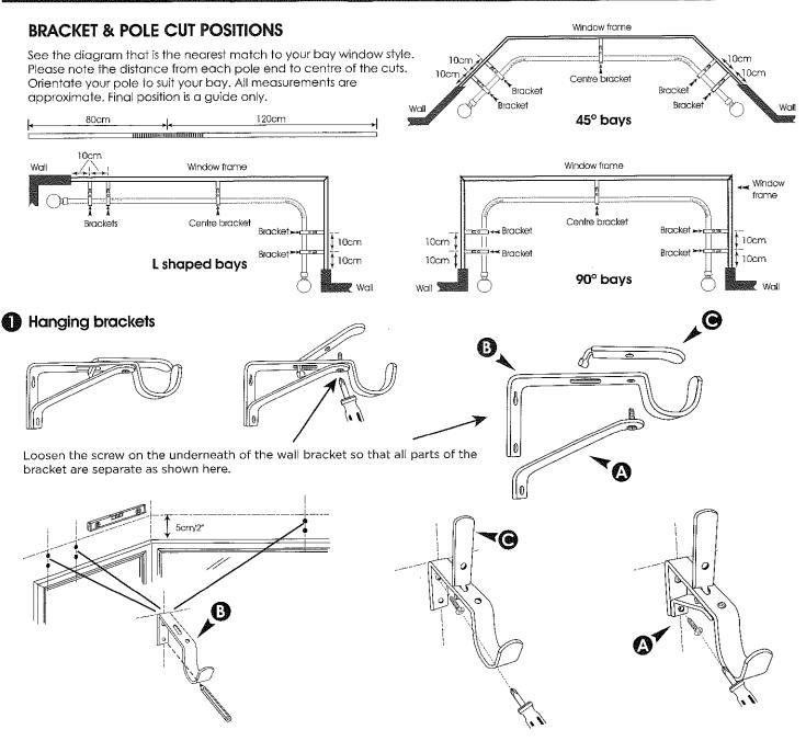
Using part **(B)** of the wall bracket, mark the drill holes on the wall at the required position. Check they are all level.
