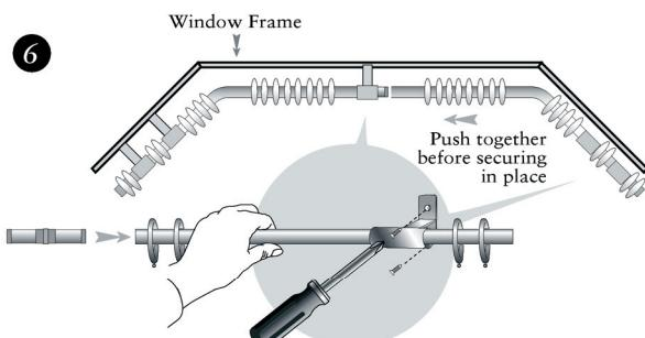
6. Insert the joining splice into the second pole and again using 2 persons, push the 2 poles together before securely fixing to the wall or ceiling.
