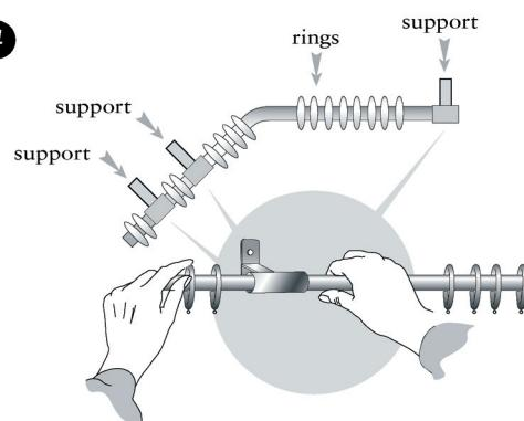
4. Slide 1 ring for every 10 cms of pole and 2 supports onto both poles and one in the centre as diagram above shows ensuring 2 rings are placed between the two end supports. 1-2 rings should also be allocated for the space between the end support and the finial. Allow the supports to hang loosely from the pole at this stage.
