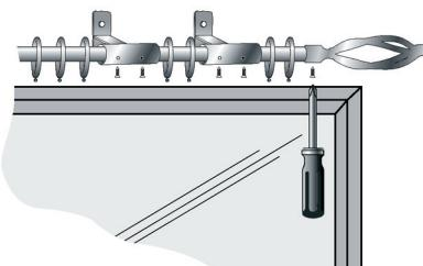
7. Tighten the grub screws in the supports to hold the pole in place and fix the finials, ensuring 1 or 2 rings are between each end support and finial, these will act as end stops.
