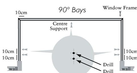
1. Mark and drill the positions, (using a 6mm drill bit), for the 5 supports as shown by arrows in the illustration that best matches your window. Ensure the Centre Support is positioned in the middle of the window. Insert the wall plugs supplied.
