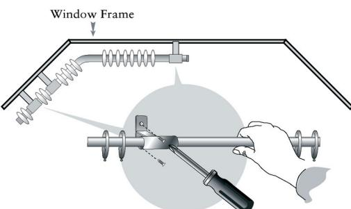
5. Whilst 1 person holds the pole in position, the other person should securely fix the complete set in place to the holes drilled in Step 1.
