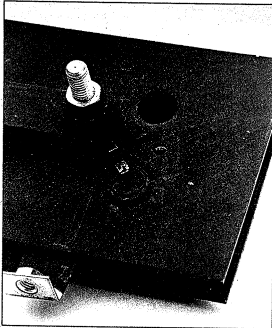
(Fig. 14) Shorted Diode in Rectifier
