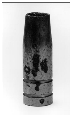
Figure 9 Spatter Build Up Symptoms
