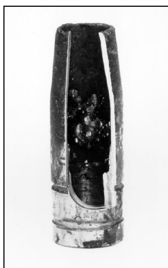
Figure 10 Spatter Build Up
