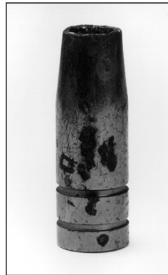
Figure 9 Spatter Build Up Symptoms
