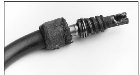
Figure 12 Spatter Damaged Swan Neck
