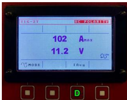
Fig. 7; By pressing button D (Fig. 11) while welding, you can toggle between displaying the average amperage and the max amperage.
