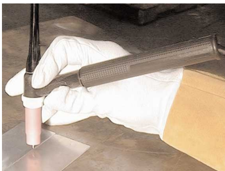
Fig 10 – Holding the TIG Torch
