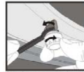
4 Tighten anti-thief nut by wrench with reverse
