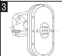
POSITION THE FIXTURE over the fixture screws and secure in place with thumb nuts (provided). Fixture may be mounted orientated down when the fixture is mounted to a wall.
