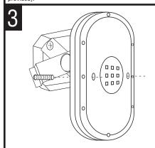
POSITION THE FIXTURE over the fixture screws and secure in place with thumb nuts (provided). Fixture may be mounted to ceiling or wall. The photo sensor or knock out must be orientated down when the fixture is mounted to a wall.
