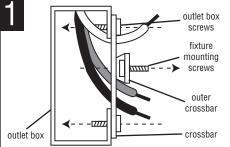
THREAD fixture mounting screws (provided) into outer cross
