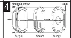
PLACE DIFFUSER ON CANOPY. Then place bar grill or frame over diffuser and attach to canopy with mounting screws (8-32x1/2, 4 combination head screws provided). NOTE: On models with hood, attach diffuser to base with one combination head mounting screw at center top of base only. Place hood over diffuser and secure to base with remaining three mounting screws.
