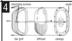
PLACE DIFFUSER ON CANOPY. Then place bar grill or frame over diffuser and attach to canopy with mounting screws (8-32x1/2, 4 combination head screws provided). NOTE: On models with hood, attach diffuser to base with one combination head mounting screw at center top of base only. Place hood over diffuser and secure to base with remaining three mounting screws.
