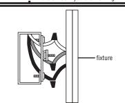
CONNECT THE WIRES. NOTE: Attach black fixture wire to black supply wire, white fixture wire to white supply wire and green fixture ground wire to ground wire in outlet box. NOTE: wire connectors not provided. NEVER CONNECT GREEN FIXTURE GROUND TO BLACK OR WHITE POWER SUPPLY LEADS.
