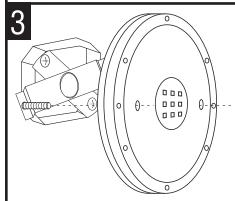
POSITION THE FIXTURE over the fixture screws and secure in place with thumb nuts (provided). Fixture may be mounted to ceiling or wall. The photo sensor or knock out must be orientated down when the fixture is mounted to a wall.
