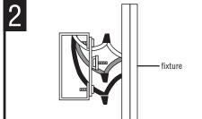
CONNECT THE WIRES. NOTE: Attach black fixture wire to black supply wire, white fixture wire to white supply wire and green fixture ground wire to ground wire in outlet box. NOTE: wire connectors not provided. NEVER CONNECT GREEN FIXTURE GROUND TO BLACK OR WHITE POWER SUPPLY LEADS.
