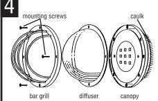
PLACE DIFFUSER ON CANOPY. Then place bar grill or frame over diffuser and attach to canopy with mounting screws. (8-32x1/2, 4 combination head screws provided)
