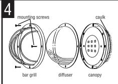
PLACE DIFFUSER ON CANOPY. Then place bar grill or frame over diffuser and attach to canopy with mounting screws. (8-32x1/2, 4 combination head screws provided)
