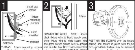
(provided) into outer cross bar. POWER SUPPLY LEADS. outlet box screws (not provided)
