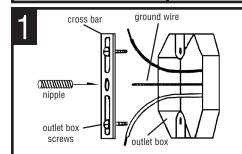
ATTACH cross bar to outlet box with outlet box screws (8-32 x 1/2, 2 slotted screws not provided)
