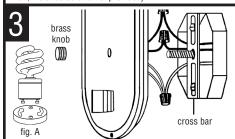
POSITION THE FIXTURE over the nipple and secure in place with brass knob. Insert lamp(s) into lampholder(s). Align and insert the round ended pins on the bottom of the self ballasted lamp into the circular opening in the lamp holder key hole slots, see figure A. Grasp the base and rotate clockwise. Be sure to use SBCFL with wattage no greater than specified for this fixture.
